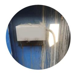
The tilt sensor is equipped with wired power supply and data transmission by default, and a wireless communication module is also optional. It can also monitor multiple inclinometers in a single device, and can detect up to 200 inclinometer data at the same time. The entire monitoring system supports the use of solar panels for power supply, and the data interface supports secondary development.
